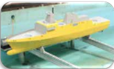
A. Ulbertus , Sideways launching process of a ship using the Arbitrary-Lagrangian-Eulerian approach
