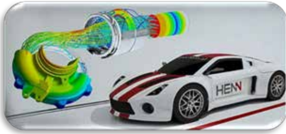
Fig. 1: Composite image from fluid, structure and acoustic analyses of a muffler connected between a turbo charger and an automotive pipe. Streamlines colored with velocity, walls with pressure or deformation and iso-surfaces from sound pressure level.
