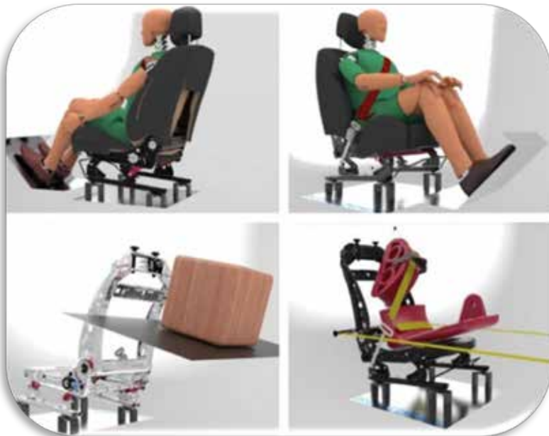
Fig 1: Four severe seat load cases at high speeds, top left is a front crash, top right is a rear crash, bottom left is a 18kg luggage crash, and bottom right is seatbelt anchorage test.
