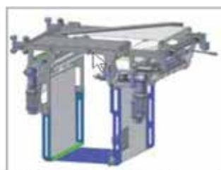
Fig. 9 - Overview of the RecurDyn model of the film feeder including flexible bodies ...
