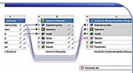
Combining Static and Harmonic Stress Analyses for Fatigue Assessment Using Ansys and nCode DesignLife
