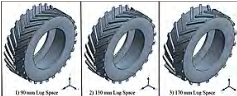
Fig1. Three-dimensional tire model in isometric and front views showing different lug spacings.
