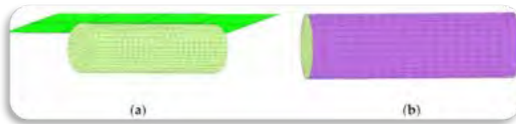
Fig. 8. FE model of the battery cell: (a) volume model in contact with a barrier, (b) battery model composed of the jelly roll volume and a case
