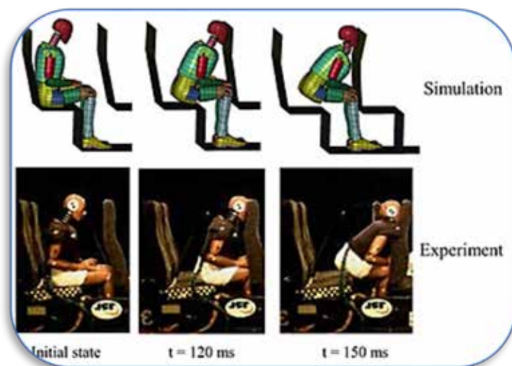
Figure 3. Comparison of dummy collision test and simulation model in seated position
